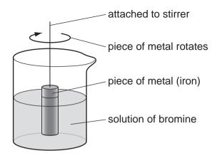
(a) A piece of iron was weighed and placed in the apparatus. It was removed at regular intervals and the clock was paused. The piece of iron was washed, dried, weighed and replaced. The clock was restarted.
